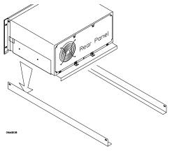
**3** Fasten the support shelf to the rack cabinet by installing the rack cabinet screws through the front support shelf ears into the cabinet rails. Use the rack cabinet hardware.
